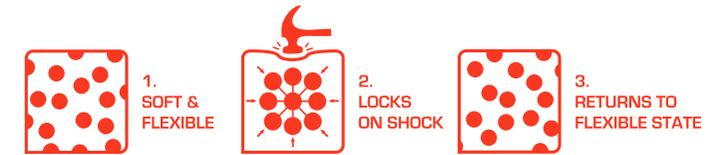
The raw material is strain rate sensitive meaning; the harder the impact, the more the molecules react, the better it protects. Another great feature of D30®, compared to many other impact absorbing products in the market, is the 100% repeat function.
