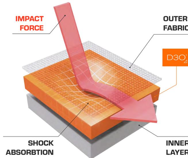
In standard conditions, the molecules flow freely allowing the material to remain soft and flexible. On impact, the molecules lock together to absorb impact energy and reduce the force transmitted. The molecules instantly return to their flexible state after impact.
